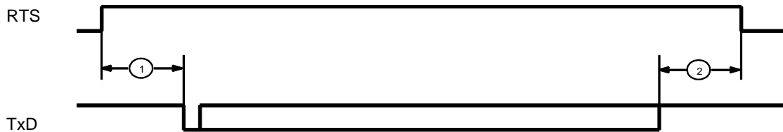
Figure 9.5-3: Transmit Timing, XCTS constant log. '0'
